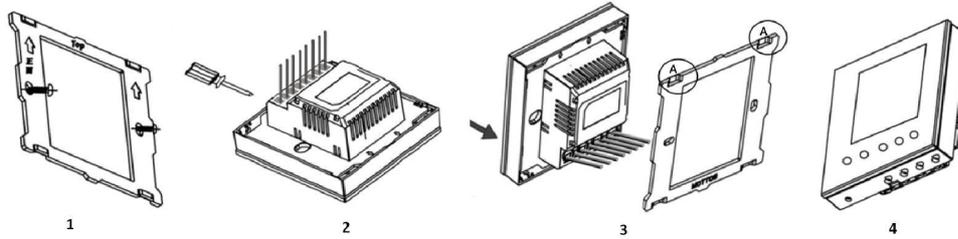
Step 1: Remove the steel frame from the device, and secure it onto the junction box with two screws.
