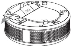
3. Remove the paper strip protecting the battery.
