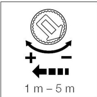
Reach is the term used to describe the radius of the detection zone produced on the ground when mounting the light at a height of 2 m.
